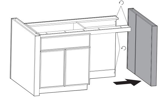
Insert refrigerator. With the unit near its final position, slide the refrigerator into place. The leveling feet on the bottom of the refrigerator can be used to tune the fit and stability. Guide the refrigerator power cord into the wire management hole on the inside of the case.
