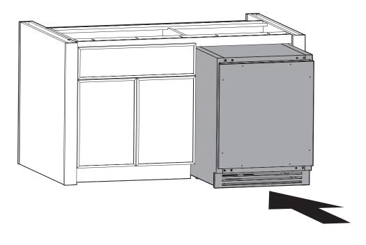
After positioning the refrigerator in its final position, rotate the two plastic anti-tip discs until they press firmly down onto the refrigerator. These discs prevent the refrigerator from tipping forward during use.
