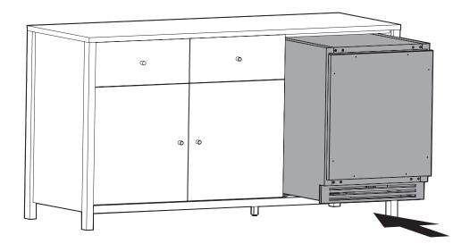
Note: If necessary, adjust leveling foot under center of cabinet
