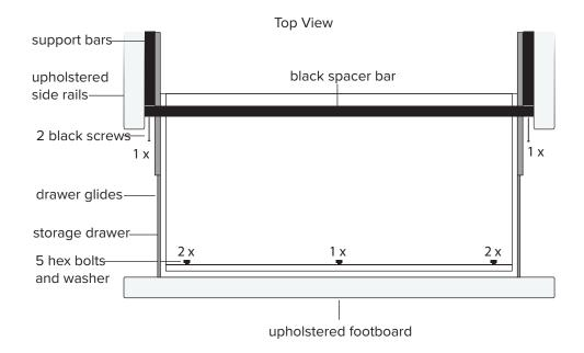
Align the holes in the glides with the pilot holes in the drawer so that glides are flush with the drawer box. Insert the eight screws from the included packet into the holes (four per side) and tighten to secure. Close drawer.
